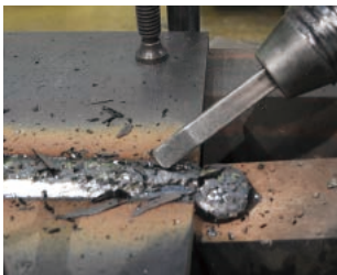
Slag removal by air chipper
