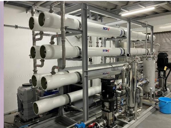
Wastewater recycling system of high recovery rate for linen laundry operations (combination of MF and RO methods)
