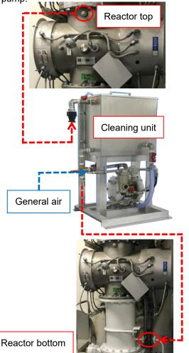
(3) Supply fresh water to the tank of the cleaning unit until the water supply is stopped by the ball tap.
