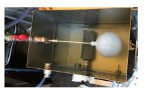
(4) After filling the tank with fresh water, switch flow path of the cleaning unit to the cleaning unit side and operate the air drive pump to circulate the water until the tank water level stabilizes for about five minutes. \*The water level can be adjusted by the air regulator supply pressure.
