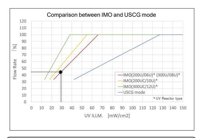
How to read the graph (Example: IMO (300U/08U) \*Red line in the graph) When the UV ILLM. (UV illuminance) is 30 mW/cm<sup>2</sup>, the Flow Rate should be adjusted to approximately 45% to prevent the "UV Dose Lower" alarm from being issued.
