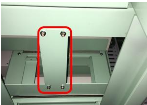
Figure 13 Attachment of rail connecting plate
