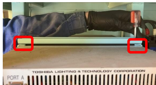
Figure 5 Removal of screws that are securing UV power unit holding plate
