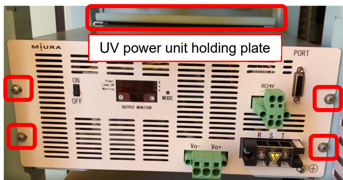
Figure 15 Attachment of 8 kW power unit fixing screws and UV power unit holding plate
