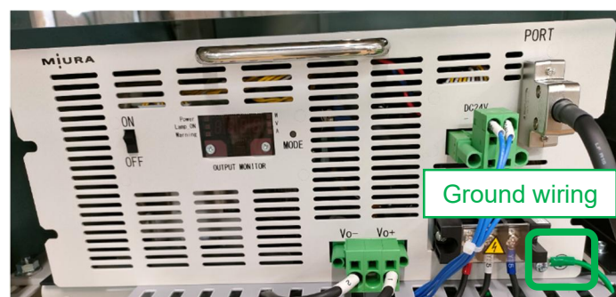
Figure 25 Wiring point on front of 8 kW power unit (ground wiring)
