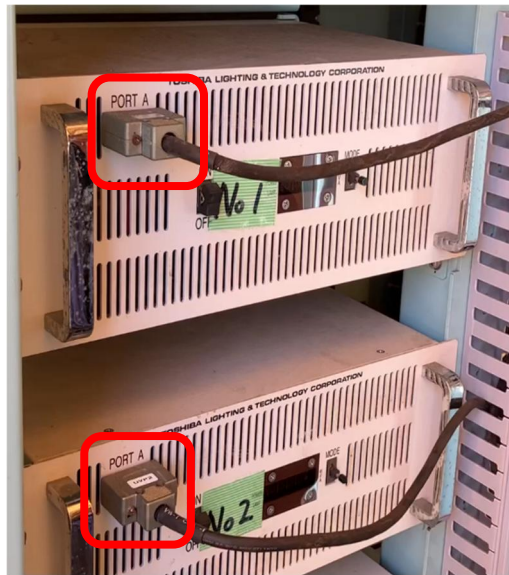
Figure 4 Connecting cable removal
