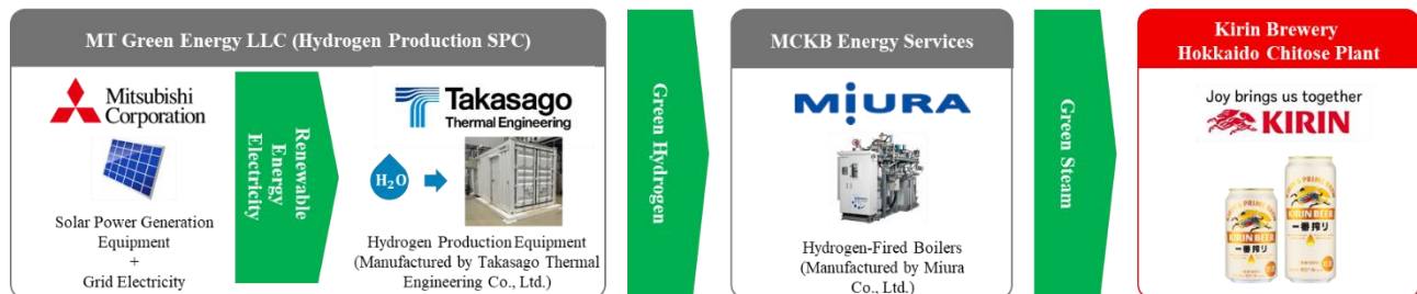
Scheme of the Demonstration Project
